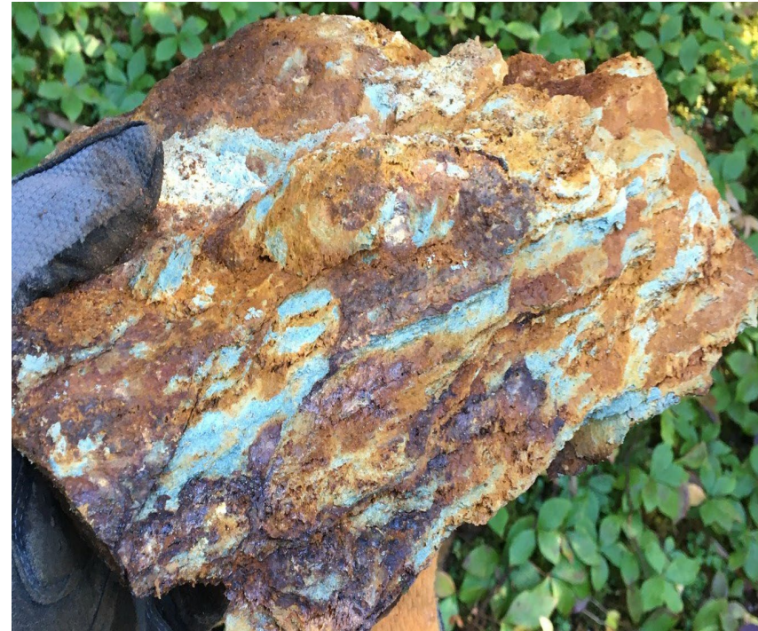
Sericite + pyrite Type Mineralization associated with the Cabot Prospect
